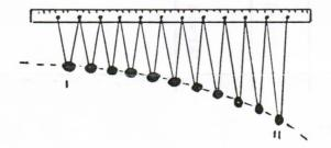
A piece of duct tape encircles each ball and a length of string passes under the duct tape and is attached to the half-metre rule with the bolts, washers and wing-nuts through holes drilled for the purpose. Hence, each ball is supported in such a way that it will swing with no elliptical motion; the length of its supporting string may be easily changed by loosing the appropriate wing-nut. I support the whole thing on any handy shelf or table leg with the C-clamp.
